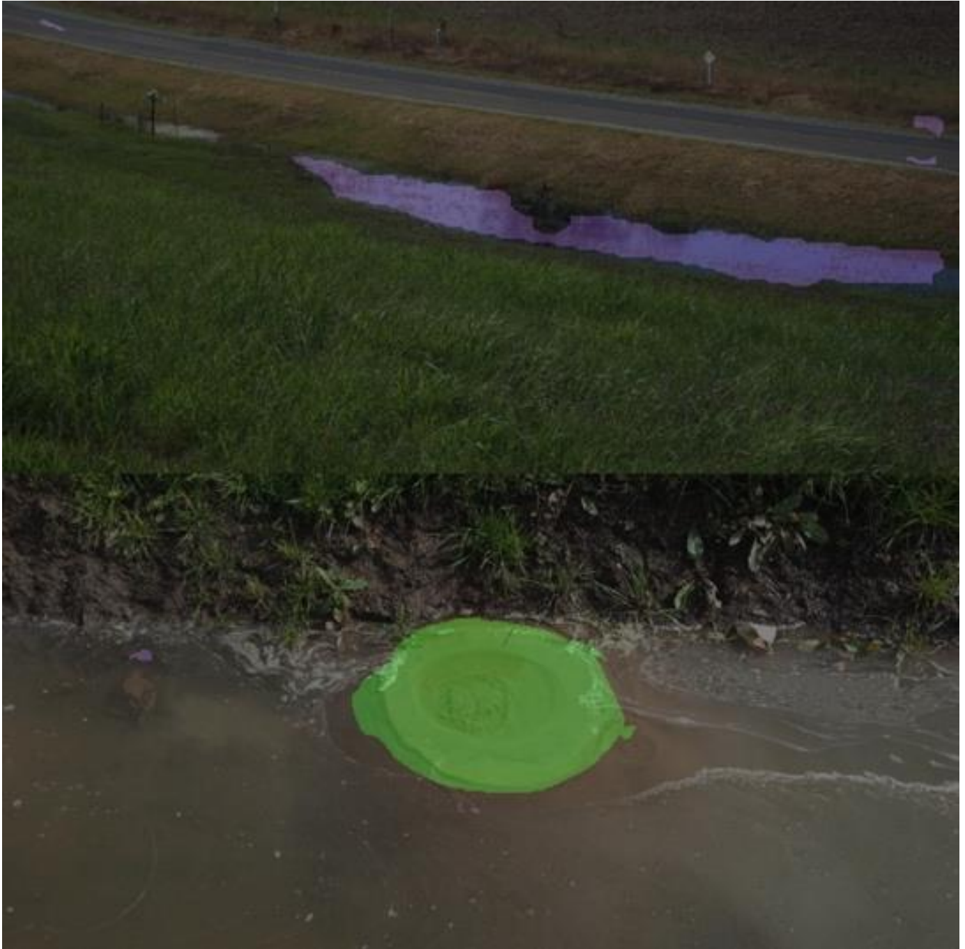
Figure 4.6: Segmentation overlay visualization from the deployed web application showing simultaneous detection of sand boil (green) and seepage (pink) defects with clearly separated masks and no overlapping, demonstrating effective multi-defect segmentation and priority-based overlap resolution.
