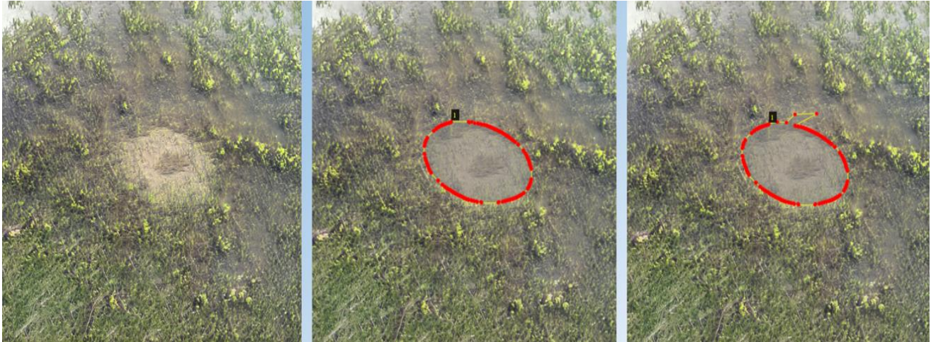
Figure 3.9: Manual adjustment of convex hull annotations using the VGG Image Annotator (VIA). From left to right: (a) the original synthetic image showing a sand boil defect, (b) convex hull-based auto-annotation visualized as a red polygon, and (c) human refinement by dragging the polygon points for precise defect boundary alignment.
