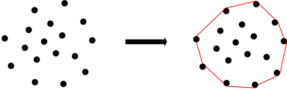
Figure 3.8: Illustration of the Convex Hull Algorithm applied to a finite set of points. The convex hull (highlighted in red) represents the smallest convex polygon encompassing all given points. In image segmentation, this concept is leveraged to automatically generate precise annotations by identifying and encapsulating the spatial extent of defect regions.
