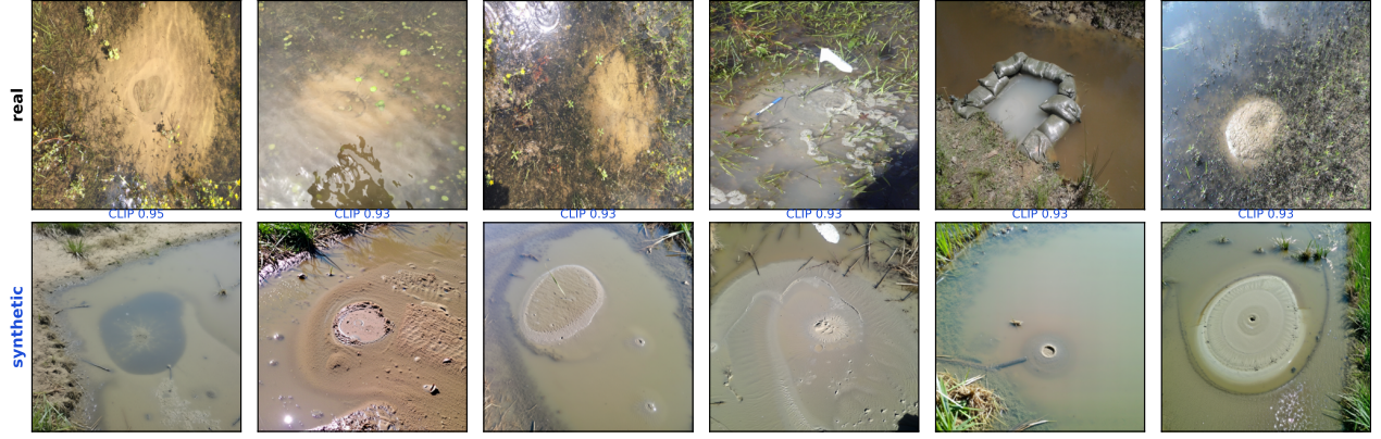
Fig. 3. Real sand boils (top) beside their best-fidelity synthetic descendants (bottom), produced by the companion generation paper [5] and carried here in the source-tagged augmented mix. Each bottom tile is the V_4 -preset descendant scoring highest under CLIP image similarity to the parent above it, and each carries a source_image_id pointer to that parent, the field on which the filter of Section III-F1 keys.
